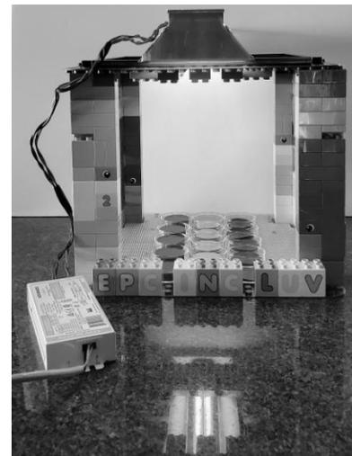
Duplo© lab setup with substrate discs and 254 nm LUV™ light fixture.
